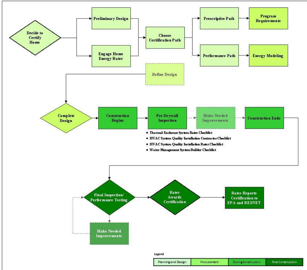
Figure A.1: Energy Star Process Flow
