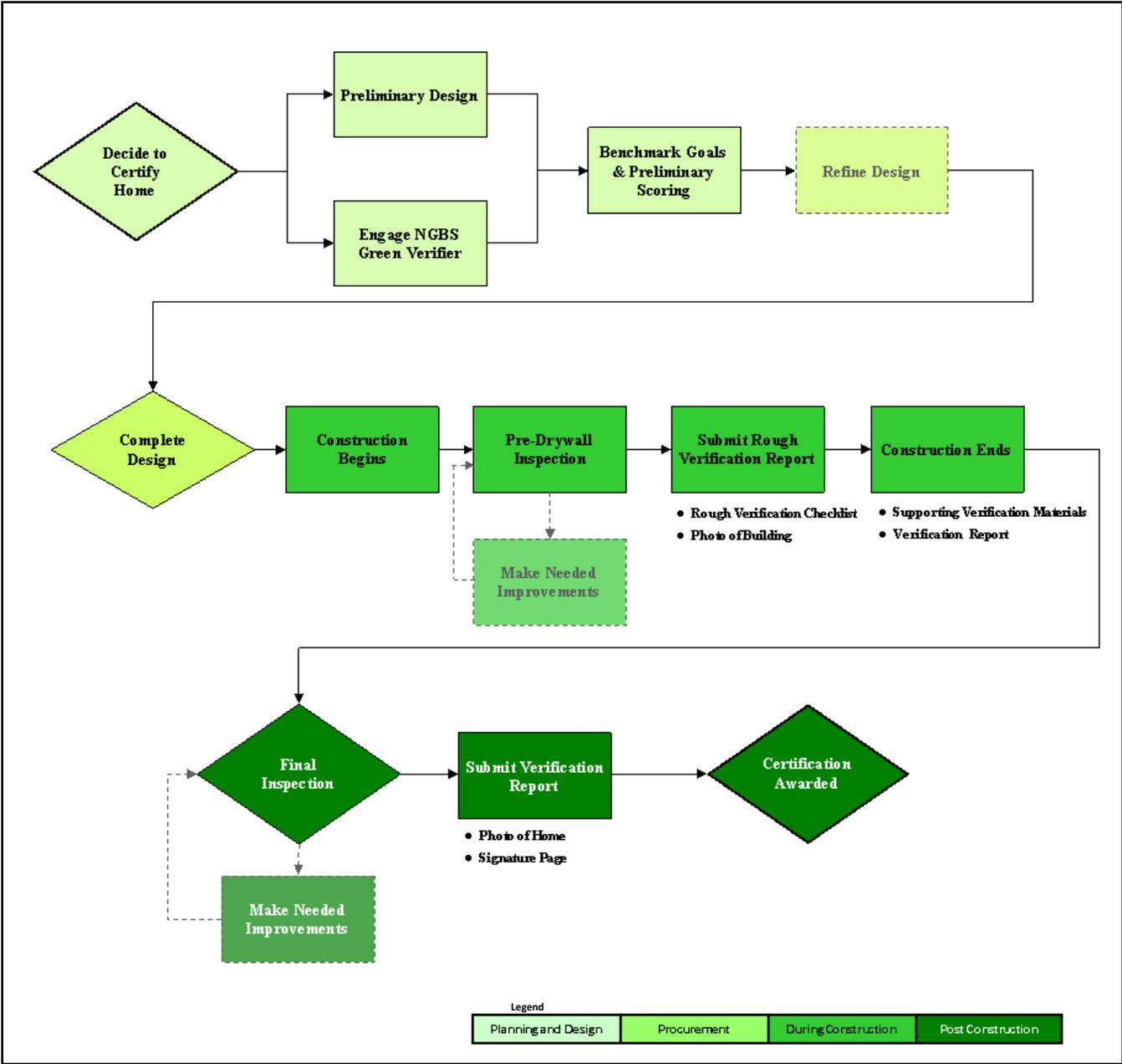
Figure A.3: National Green Building Standard Process Flow
