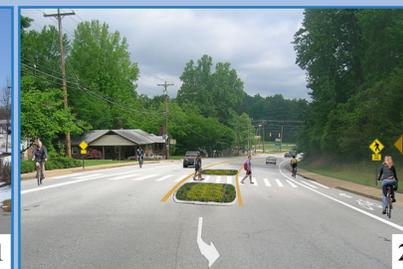
Image 1 shows a block of southbound Gratiot that does not provide pedestrians with a mid-block crosswalk. Midblock crosswalks reduce the distance a pedestrian has to travel to reach a safe or signalized crosswalk. The image also shows that there are inadequate facilities to accommodate non-motorized transportation options. Image 2 provides an example of a mid-block crosswalk option with non-motorized transportation options in Easley, SC.
